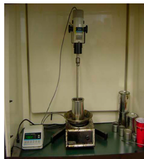
Figure 2. Mechanical mixer for stirring base asphalt with graphene platelets.
